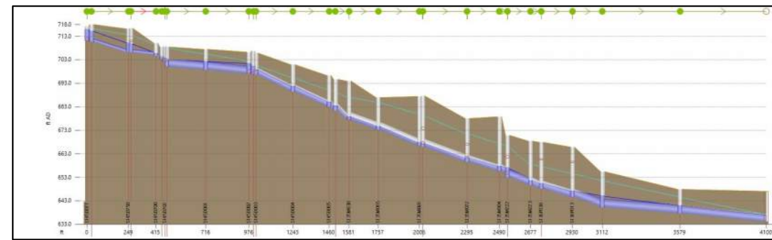
Figure 4.4.2.1 Predicted Peak HGL for the 2yr, 24hr design storm - Solution 3 vs. 'Plate Removed' Scenario.
