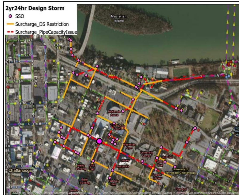
Figure 3.4.2. Predicted Pipe Surcharge and SSO for the 2yr24hr Design Storm
