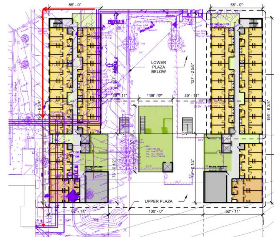
Figure 1 – Proposed Dorm Footprint Overlaid on Existing Site Utility Plan
