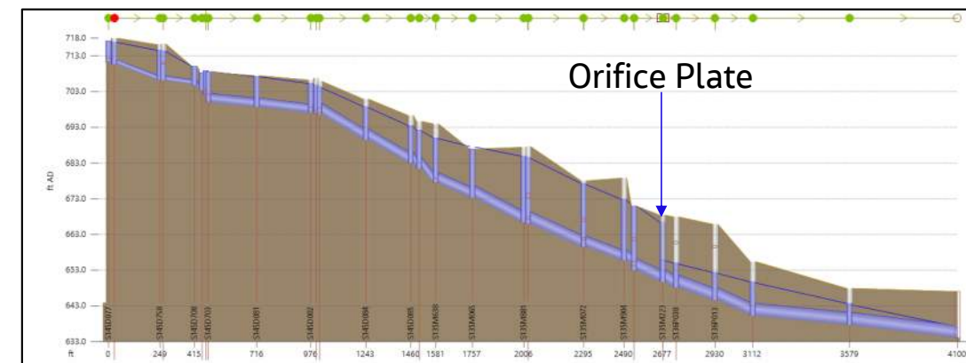
Figure 3.2.1. Predicted Peak HGL for the Jun 28, 2018 Storm Event under 'Existing Conditions' Scenario
