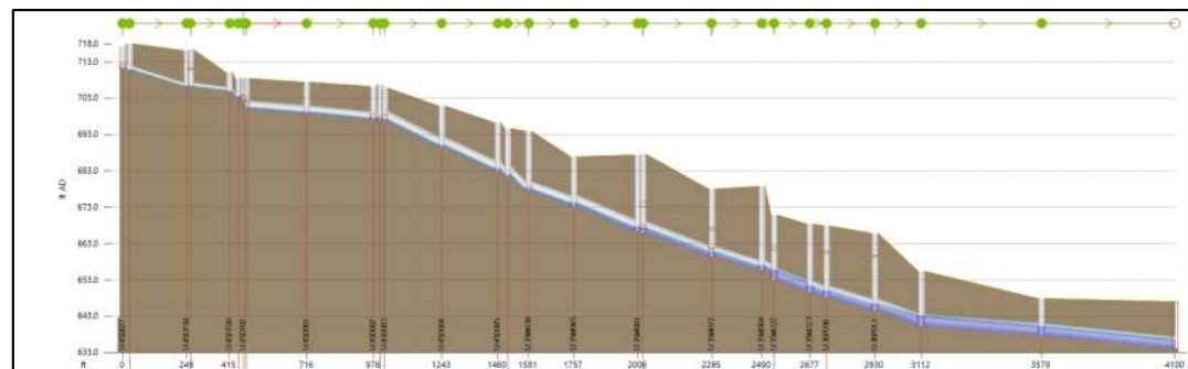
Figure 4.3.2.2. Predicted Peak HGL for Solution 2 - 5yr, 24hr vs. 2yr, 24hr design storm
