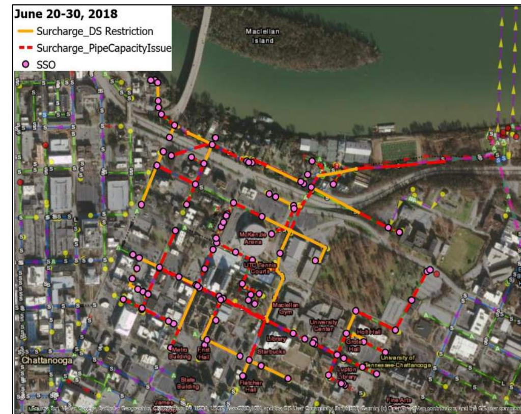
Figure 3.2.2. Predicted Pipe Surcharge and SSO for the Jun 28, 2018 Event under 'Existing Conditions' Scenario
